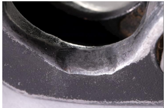
6. Deformed attachment hole
